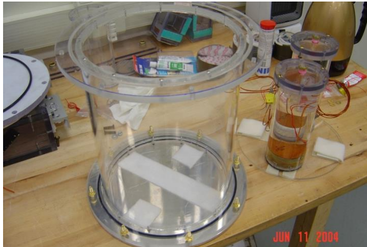
Figure 3: The Outer Containment Tank
